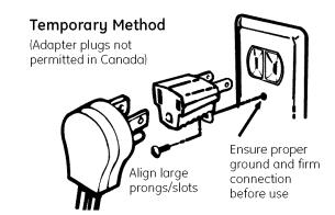
**CAUTION** — Attaching the adapter ground terminal to the wall receptacle cover screw does not ground the appliance unless the cover screw is metal, and not insulated, and the wall receptacle is grounded through the house wiring. The customer should have the circuit checked by a qualified electrician to make sure the receptacle is properly grounded.
