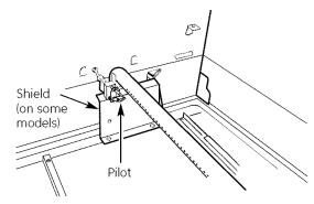
**6.** To light the oven pilot, push in and hold the oven control knob while lighting the pilot with a long match or match holder. Once the oven pilot is lit, continue holding the oven control knob for one minute before releasing.
