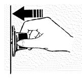
Push the control knob in and turn it to the **LITE** position (on electric ignition models) or **HI** (on standing pilot models).
