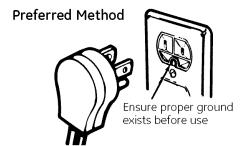
The power cord of this appliance is equipped with a 3-prong (grounding) plug which mates with a standard 3-prong grounding wall receptacle to minimize the possibility of electric shock hazard from this appliance.
