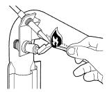
No adjustments are required for natural gas. If the range is connected to LP gas, contact the person who installed your range or made the conversion. If pilot flame does not stay lit, repeat this step.
