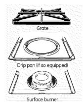
**CAUTION:** Do not operate the cooktop without all burner parts, drip pans (if so equipped) and grates in place.
