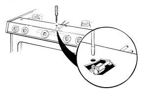
**CAUTION** — Make sure the surface burner control knobs are in the **OFF** position before attempting to adjust the pilots.
